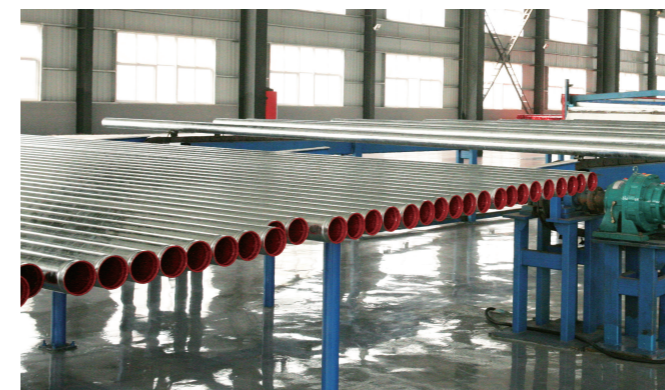
Plastic Coated Composite Pipe Production Workshop
