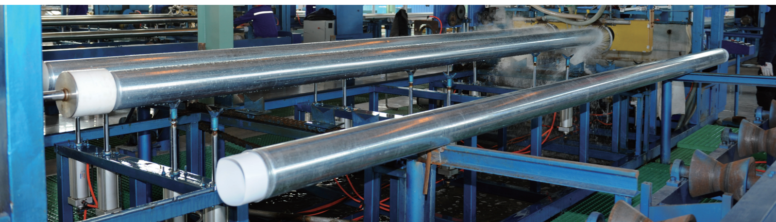
Steel Pipe of Lining Plastic Production Line
