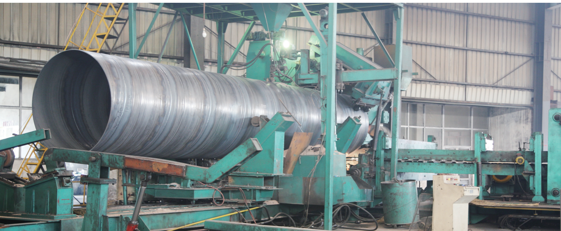
Spiral Steel Pipe Production Line
